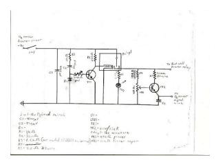
well, the main advantages of my EFIE are it's cheap and simple to build and simple to opperate/calibrate. i'm not sure the O2 sensor heater power is the best place to draw the power from, but as i said, i used it because it is only hot while the vehicle is running.
