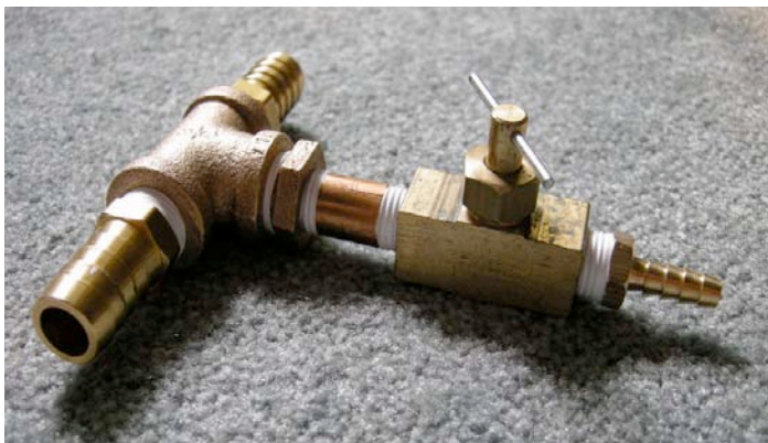
Completed adapter made out of pipe fittings with attached needle valve.
