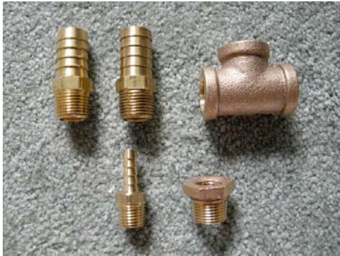
Possible parts to make a T, these are for a 5/8" heater hose. Pipe thread is 3/8".
