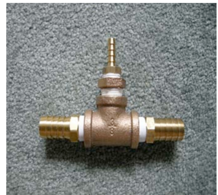
Completed adapter made out of pipe fittings.
