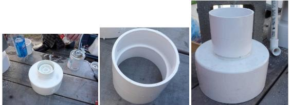
Glue the 3"x1/2" bushing onto the bottom of the 6" cap (with PVC solvent and cement); glue both flat ends together. *The 6" cap will then serve as the apparatus base and the bushing as the bottom of the main chamber*. Glue the 3" coupling onto the bushing. Apply weight to the pieces to assure a good 'weld'. Allow the glue to completely dry before proceeding with the base.
