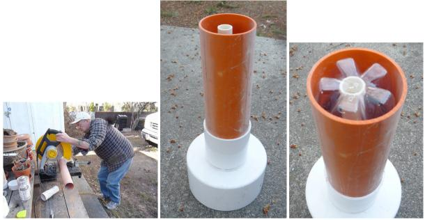
If using the 'simplest configuration' the height of the 3" PVC pipe, when fully inserted into the coupler, will be about 1/2" higher than your 1/2" gas tube so water doesn't fall out of your apparatus.
