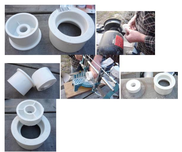
Shape the two bushings and glue them together to achieve a 3"x1/2" bushing that has a large flat surface; so it can be securely glued to the base. I shortened the inner bushing and ground off the lip, so that it would slide into the outer bushing to achieve a flat surface.
