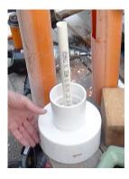
Glue the 1/2" gas pipe into the base (inserting it from the bottom). Use plenty of solvent (to soften the plastic) and glue (to assure a good seal). Make sure the 1/2" pipe will go straight up the center of the chamber.
