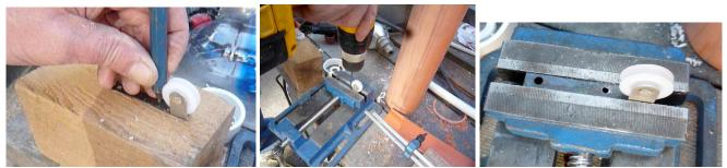
Drill appropriate holes in the pulley mounts to allow them to fasten to the cap. I pre-punch the places where I'm going to drill, or it is difficult to drill accurately in the spring steel.
