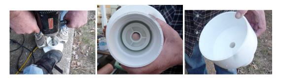
Hold the base and drill firmly so the hole does not become oblong (a drill press works well, if you have one). If the hole is cleanly made, the gas tube will be held straight. *If the hole is oblong, then it will still seal (with the glue) but you'll need to hold the gas tube straight until the glue hardens.*
