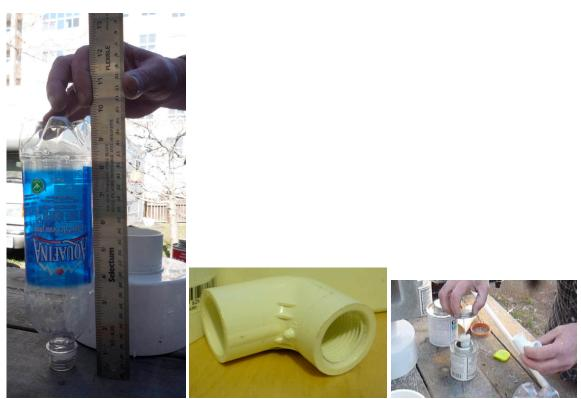
Gas tube length is the total of about 1" for the fitting, about 1" for the bushing, plus the height of your bottle (when your bottle is cut off at the 700 mL mark) and plus 1/2" for clearance (so bottle sits on the gas tube, not the bushing).
