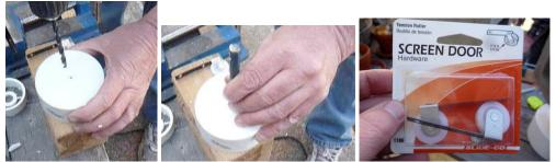
Drill, using a 1/16" drill bit, a hole in the exact center of the pulley cap, then drill the hole out to 1/4".
