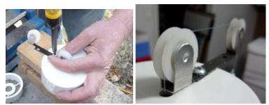
Screw the pulleys onto the cap. The edge of the inner pulley will allow a fishing line to fall directly to the middle of the bottle. *The pulley outside just needs to be far enough out to prevent the counter-weight bottle from rubbing on the 3" pipe.*
