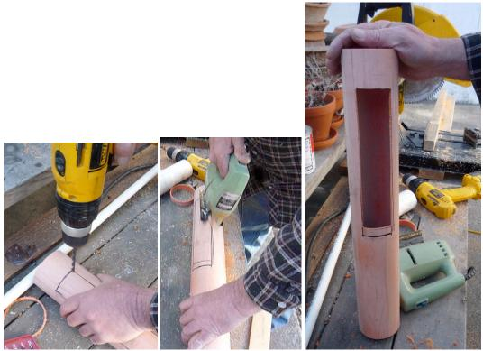
If using the counterweight option, the pipe will be about twice the height of your bottle plus 2" for top clearance.
