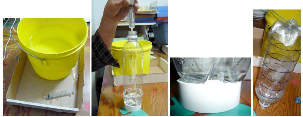
Pour water into the bottle until the water in all the 'stand holes' is even with the rise in the center of the bottle. *This is to eliminate the inaccuracy caused by this 'excess' volume that will not fill with water when the bottle is on the stand pipe.*
